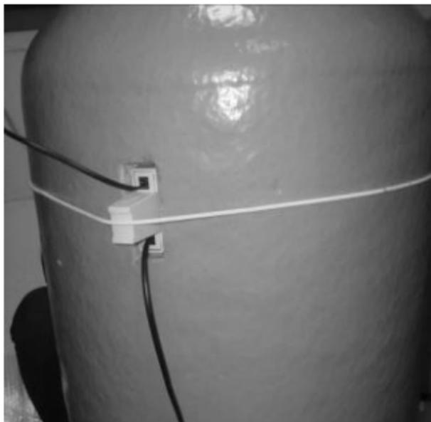
For a daisy chain installation of pipe/ tank sensors, it is important that you do not disturb the slider button positions, otherwise none of any SES 002 sensors will communicate.
