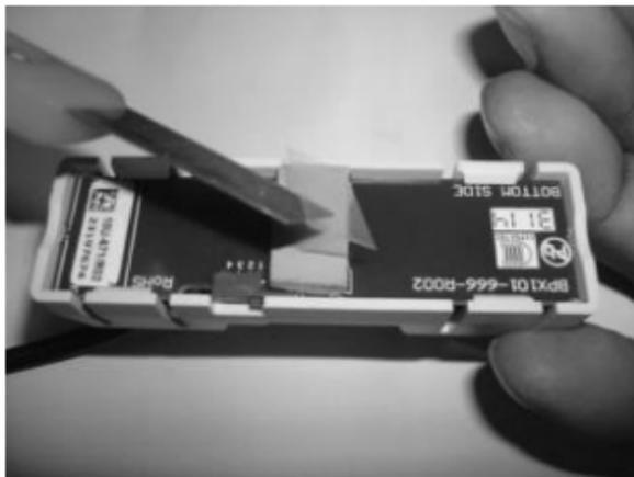
Attach the RJ10 cables and carefully insert tank sensor into uncovered space, which you prepared earlier. Keep the thermal conductive pad towards the copper pipe/ boiler tank and press gently and gradually until it appears stable over the installation surface.
