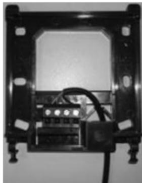
Make a communication cable entry path in back side of SES 302/ SES 303 by cutting thin plastic wall as shown below:
