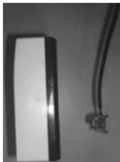
After successful inclusion of all SES 002/ 003 with SES 302/ SES 303 in the formed chain, detach the four-pin black, female connector carefully from the four-pin metallic
