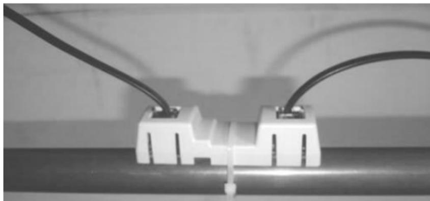
Up to four pipe or tank sensors can be daisy chained in this manner. Each sensor must have a unique logical address, set in an increasing order from hardware address 1 (e.g. if you have only 2 external sensors these must have address 1 and 2, not 3 & 4, 1 & 3, 2 & 3 or 1 & 4) otherwise the SES 302/ SES 303 will not detect them. The address is set by sliding the side button on each sensor.
