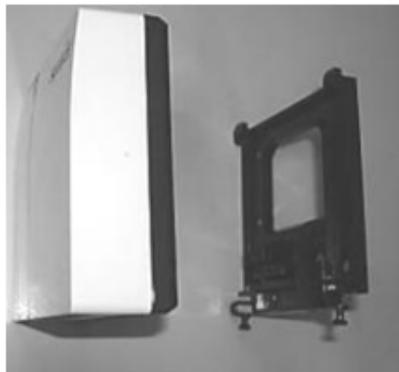
The back plate has a four-pin electrical connector. The connector block can be removed from the back plate by releasing the locks on the reverse side of the plate. A flat screwdriver will
