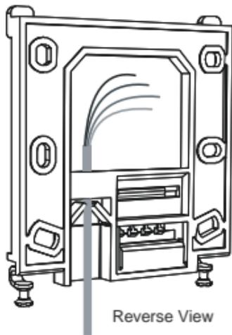
Refer to the diagrams above. Feed the stripped end of the RJ10 cable through the cable guide (see reverse view). Pull through a sufficient working length of cable.
