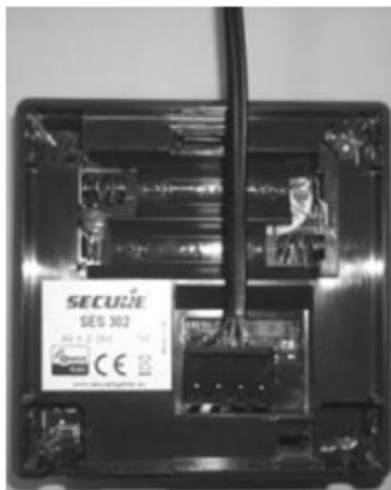
Now insert RJ10 end of this telephone cable into the pipe/ tank sensor (either socket). The other socket can be used to connect with a second pipe/ tank sensor (daisy chain). The second telephone cable with RJ10 connectors at both ends is supplied for this purpose.
