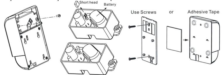
3. Knock out the thin wall on the bracket. Power line goes through the hole on bracket and connects to screw terminal on ZM1602.
