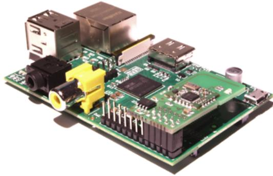
Thank for you buying **RaZberry** that turns your Raspberry Pi into a Z-Wave enabled Home Gateway. It implements the Z-Wave transceiver including the low level network protocol, the Z-Wave application level protocol and a Java Script based automation engine.
