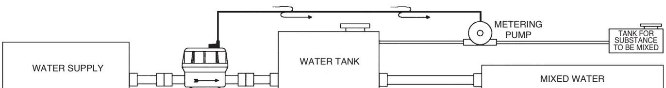
Rate of flow control: by a suitable electrical output and with addition of electronic instrumentation, several operations are possible, such as: valve and pump control, warning systems etc., according to different pre-selected rate of flow values
