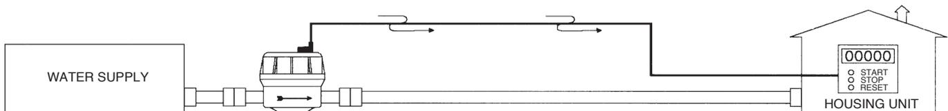
Remote reading (in combination with a remote display or a computerized reading system, it is possible to collect and process water consumption data in multi apartment buildings, where the access to water meter is often difficult, or wherever central reading of several meters is required)
